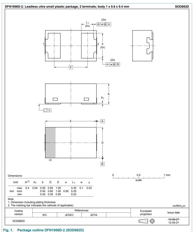
leadless ultra small plastic package; 2 terminals; 0.65 mm pitch; 1 mm x 0.6 mm x 0.4 mm body
